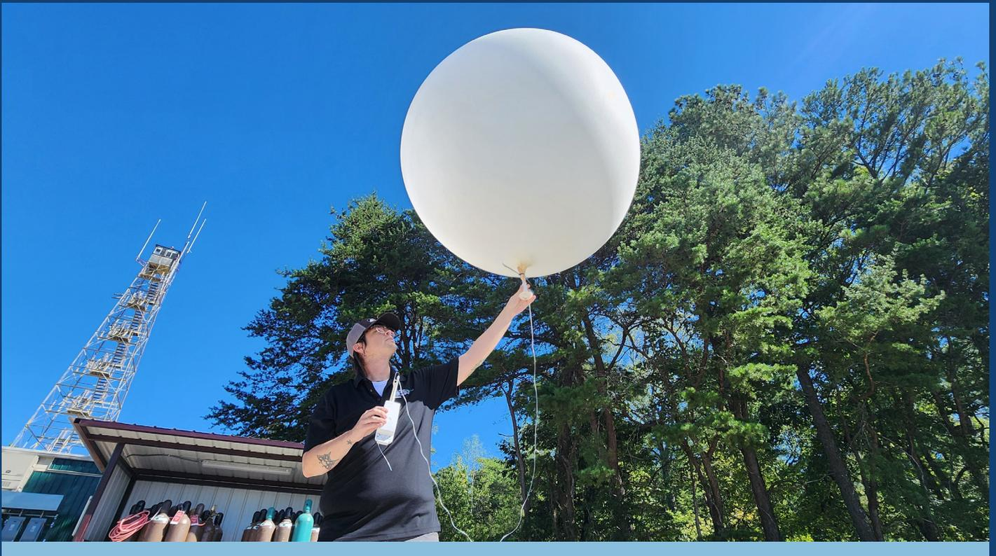
On September 18, 2024, technician Kris Bennefield prepares for a test launch of a balloon-borne radiosonde at the main site of ARM's Bankhead National Forest atmospheric observatory.
