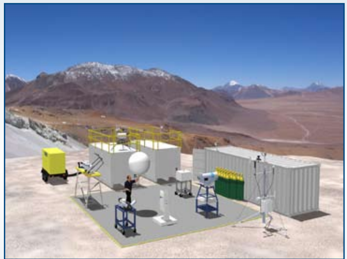
This artist's rendering illustrates a general layout of the RHUBC-II instrument suite on Cerro Toco.
