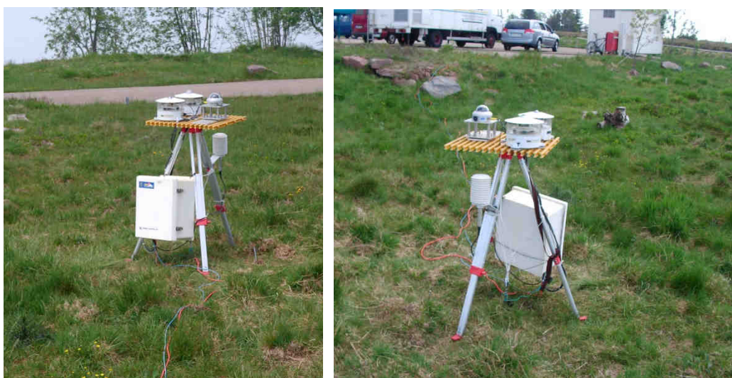
Fig. 11.29 Picture of Radiative Flux Analysis System instruments and data logger enclosure at COPS Hornisgrinde Site
