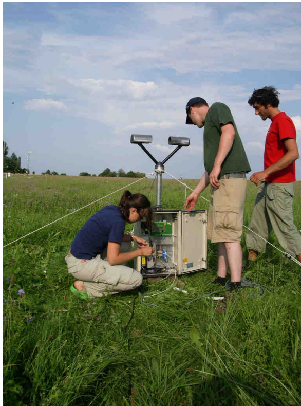
Fig. 7: Students from the University of Vienna during the installation of the distrometer.
