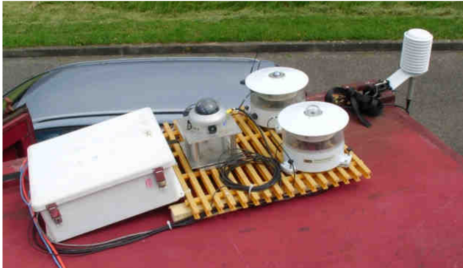
Fig. 11.54 Picture of Radiative Flux Analysis System instruments and data logger enclosure on top of the red seatainer at Supersite R,
