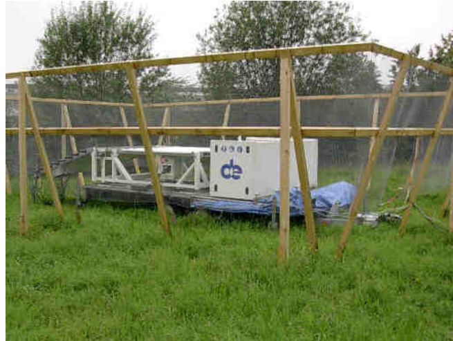
Fig. 11.50 University of Manchester Radio Wind Profiler in Achern. A clutter screen was developed in order to properly operate the instrument.
